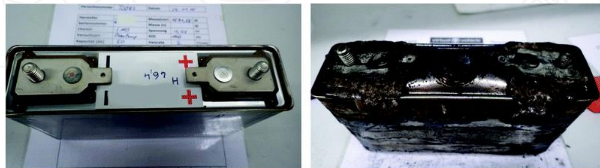
Fig 4. Tested cell before and after the thermal runaway experiment. On the fresh cell, the burst-plate of the cell is hidden below the white sticker. After a thermal runaway the cell is heavily damaged: the burst plate is open, the plastic insulation of the terminals is melted, and the cell casing is deformed by the pressure inside the cell [8].
